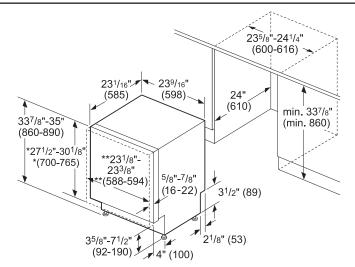
\* measured from the bottom edge of the countertop panel thickness recommended 3/4" (20 mm).
